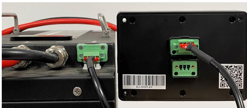
**NB:** the display only works when the battery is switched on.
